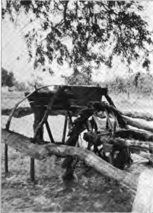
Water-wheel for the irrigation of the fields in Khiva. The current drives the wheel, raising the water in the earthenware pots placed slantingly aslope. From the wooden pipe the water runs out into the ditches in the field.
